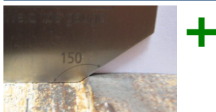
Dressed weld reinforcement
