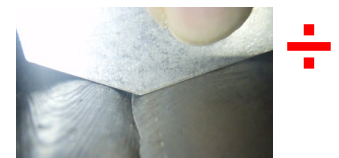
Angle approximately 130°, measured at a thickness reduced area
