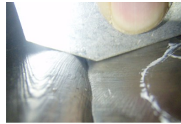
Angle approximately 110°, measured at a thickness reduced area
