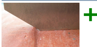
If the weld has a smooth transition, for example. Obtained by grinding, this has to be accepted.
